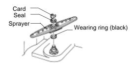
2) After the sprayer is taken off, wash out the adhered matters completely.
